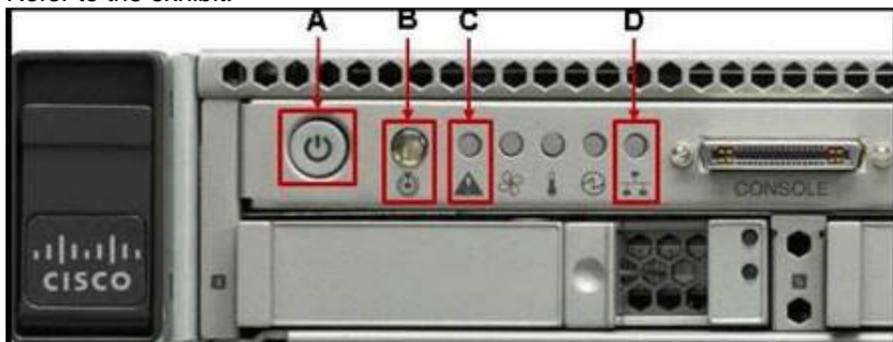
Which statement correctly identifies the front panel LEDs on the Cisco UCS C220 Server?
