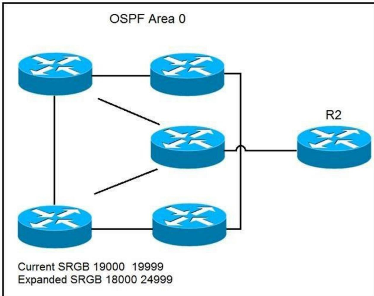
Refer to the exhibit. A network operator wants to expand the segment routing global block in upcoming maintenance. The operator must ensure that the changes to the segment routing global block have no adverse impacts on the prefix-sid associated with the loopback0 interface used within the OSPF domain. Which command can the operator use to enforce R2 to have a strict prefix-sid assignment to loopback0? A.
