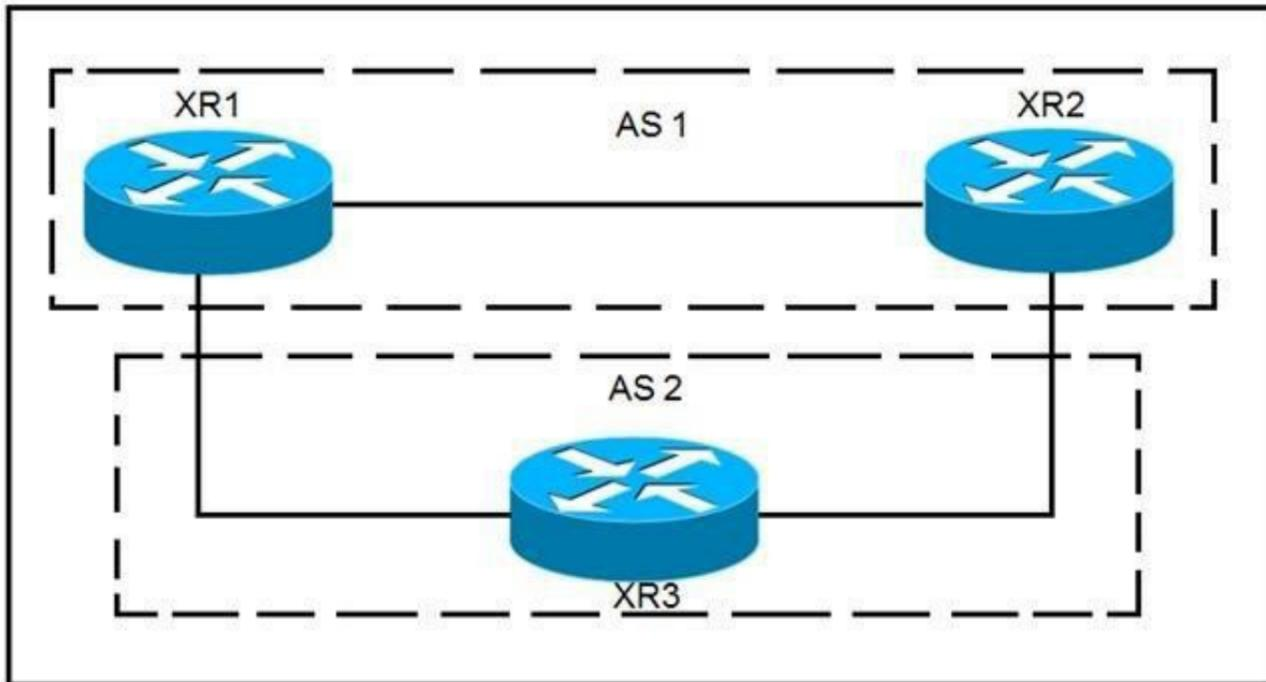
Refer to the exhibit. XR1 and XR2 are sending the prefix 10.11.11.0/24 to XR3. A configured policy on XR1 is incorrectly prepending AS path 11 11 12 12 onto this prefix. A network operator wants to add a policy onto XR3 that will not allow the falsely prepending prefix from being installed. Which policy configuration applied to the XR3 neighbor configuration for XR1 can accomplish this requirement without impact to other or future received routes?
