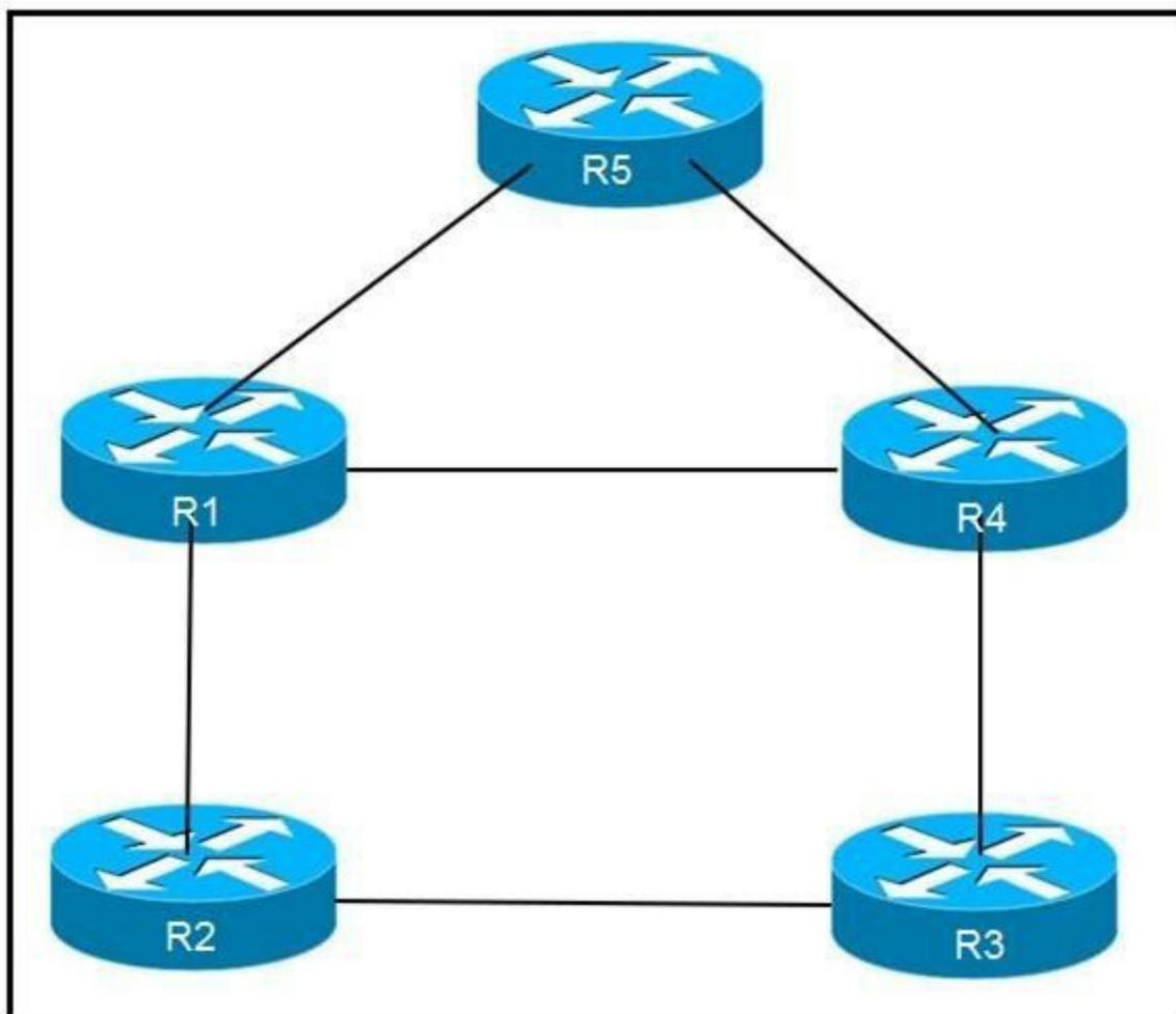
Refer to the exhibit. An engineer is addressing an IS-IS design issue which is running within the topology. All links are running on FastEthernet, except the link between R5 and R4, which is Gigabit Ethernet. Which statement about the design is true?
