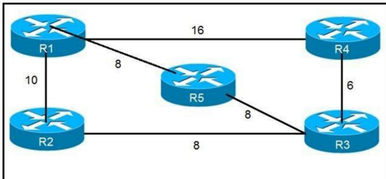
Refer to the exhibit. Which router does R1 install as an alternate next hop when trying to reach R3 if LFA is enabled?
